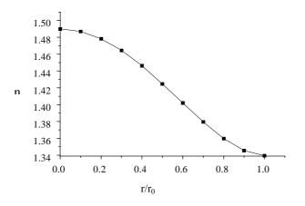
Figure 2 Ideal refractive-index profile of the GRIN sphere lenses
