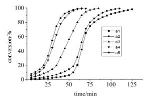
Polymerization temperature 70 , initiator concentration al ~ a5(0.5 ~ 2.5%)
